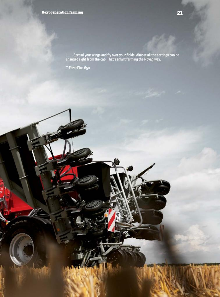
— Sheer power where it's needed. Novag T-ForcePlus no-till drills are capable of automatically adjusting their downforce to match actual soil resistance in real time
