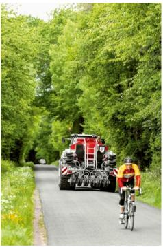
The narrow transport width of 3 m provides fast and safe transport. Further, the folding wings are automatically locked with a mechanical hook when raised for the road.
