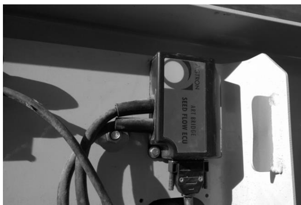
Fig. 34 : ISOBUS controller inside the main electrical box
