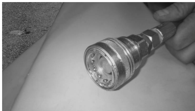
Fig. 6 : Brake hose with special coupler
