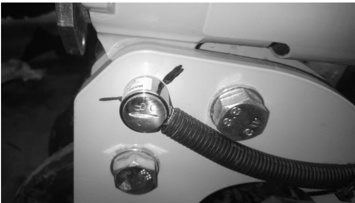
Fig. 46 : Opener with IForce sensor
