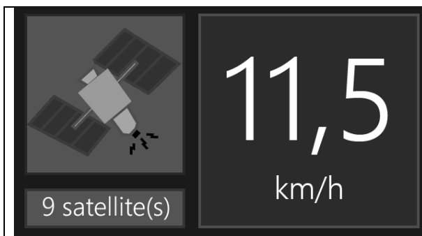
Fig. 55 : Signal quality symbol on the monitor
