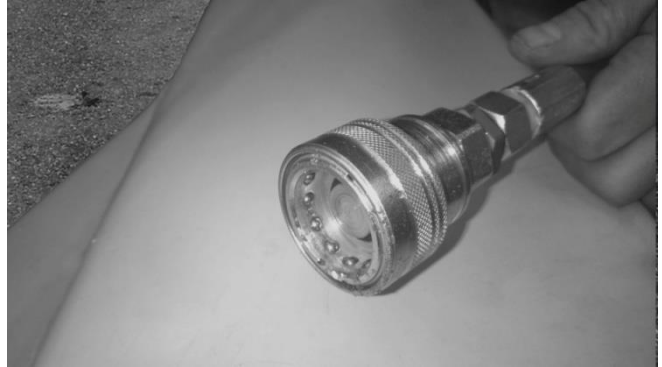
Fig. 6 : Brake hose with special coupler
