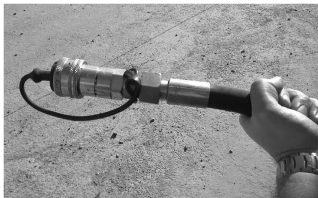
Fig. 19: Return hose on the drill
