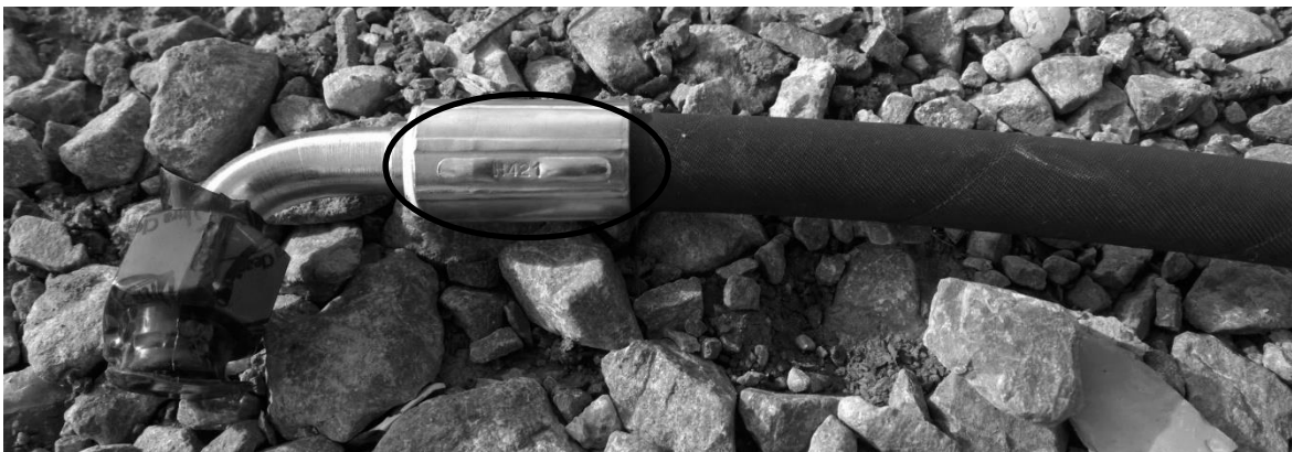
Fig. 63 : Location of ref. Nb on a hydraulic hose.
