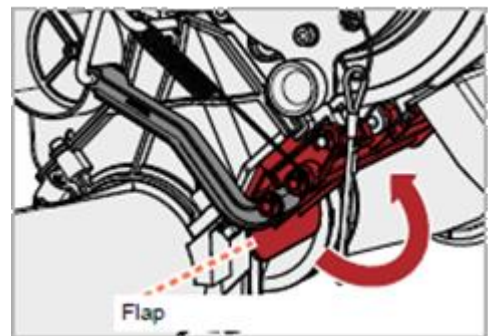
Fig. 40 : metering unit calibration flap
