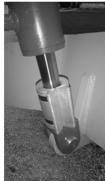
Fig. 3 : Clip kit for mounted on the cylinder
