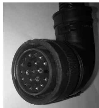
Fig. 15 : Elbow connector on the drill cable
