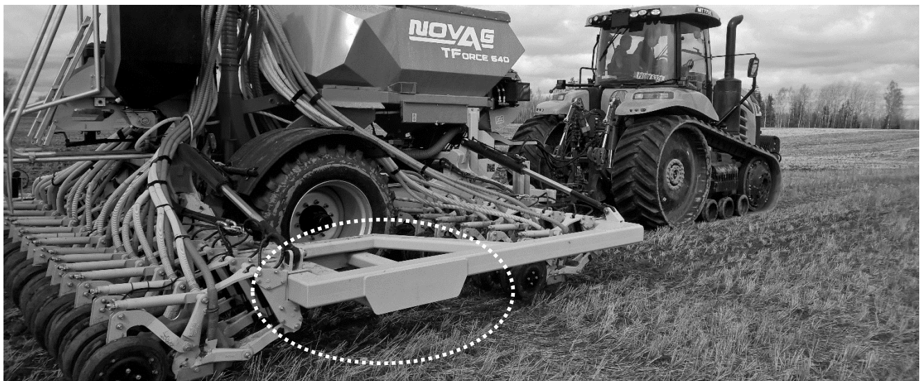
Fig. 36 : Ballast location on 6m drill
